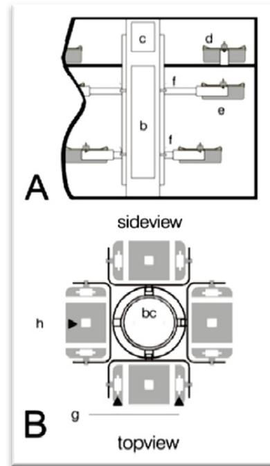
*Fig. 1 Schematic layout of the MidiCAR centrifuge.*
