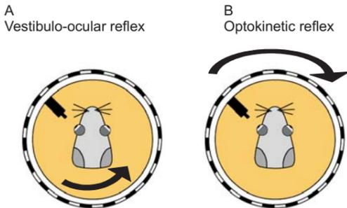
Video eye movement recording apparatus with table rotating sinusoidally during vestibular stimulation and drum rotating sinusoidally during optokinetic stimulation.
