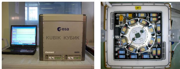
**Figure 1.** Plungerbox. A. schematic representation of an automated tissue culture module (20x40x80 mm) made of a single block of polysulphone (PSU) as it was developed by the Centre for Concepts in Mechatronics (CCM; diagram courtesy of Dr. van Loon; HW, waste or sample holder; PL, plunger; FR, fluid reservoir). B. Plunger box unit with nitric oxide (NO) sensor (arrow). C. KUBIK incubator and centrifuge facility. Pictures courtesy of Centre for Concepts in Mechatronics (CCM).
