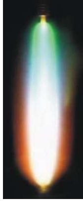
Figure 2.1: (printed in colour in figure 1.3) Picture of a HID lamp burner (real size 8 mm x 20 mm); colour separation is clearly visible.
