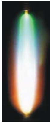
Figure 5.1: (printed in colour in figure 1.3) The burner of a MH lamp (10 mg Hg, 4 mg \text{DyI}_3 , input power 150 W). Colour segregation is clearly visible [37, 67].
