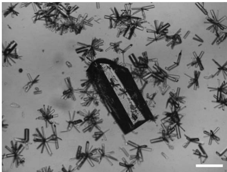
Figure 3.7: Clusters of monoclinic crystals in a 10 mg/ml, 0.1 M NaSCN, 0.05 M NaOAc/HOAc solution of pH 4.5 at 15 °C. The large crystal was seeded into the solution. The scale bar indicates 50 \mu\text{m} .
