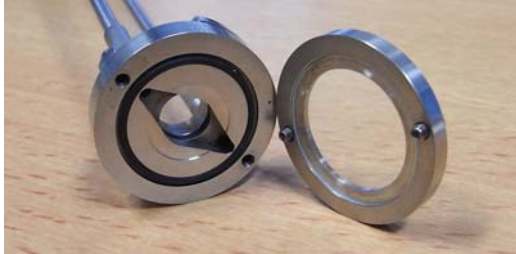
Fig. 1 Opened culture chamber that was used for experiments in the magnet. The central circle provides space for a 12 mm coverslip. After insertion of a coverslip, a glass lid was placed on top of the chamber. The two tubes at the other side of the chamber were used for fluid refreshment, allowing chemical fixation while the experiment was ongoing
