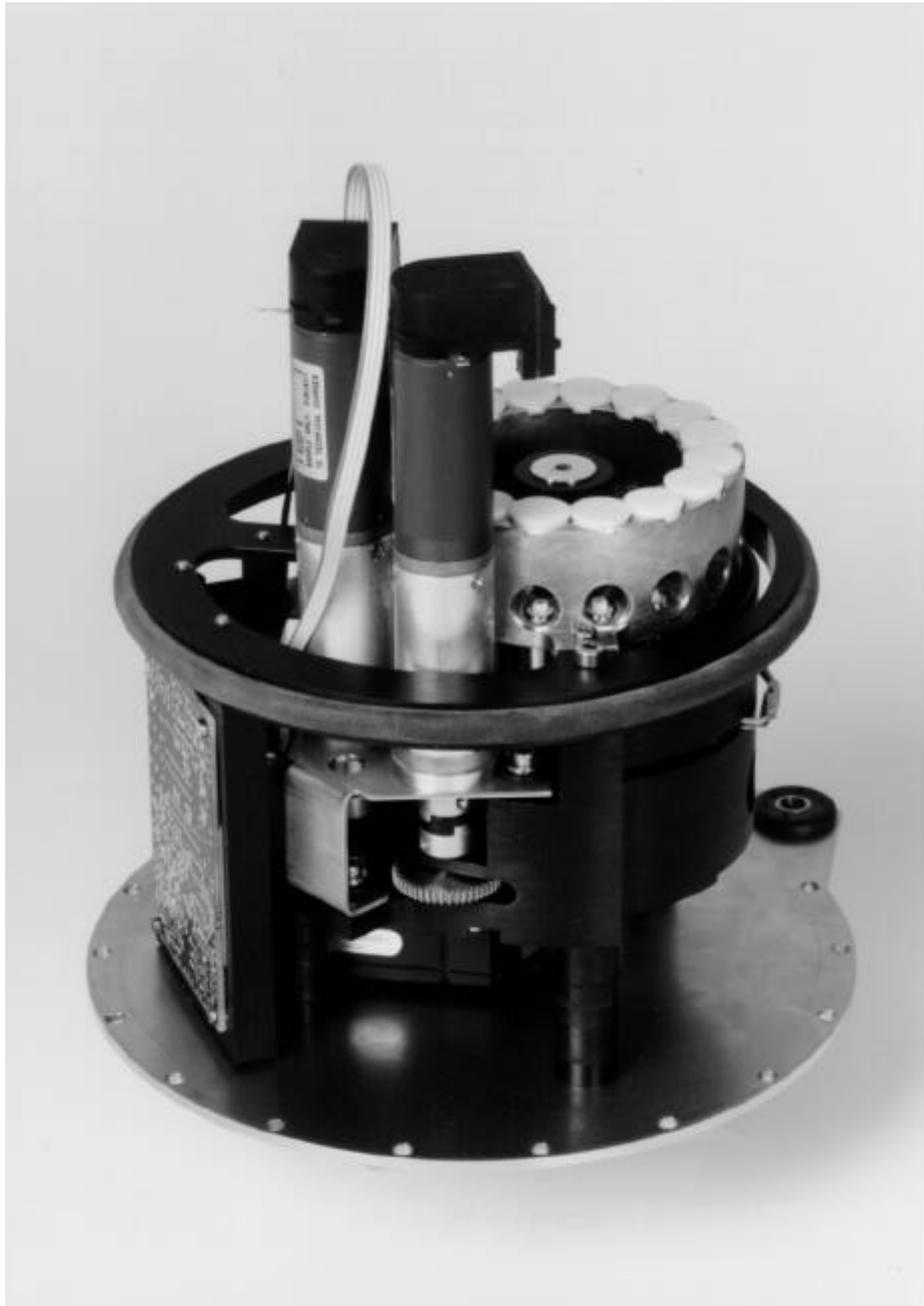
*figure Fout! Bladwijzer niet gedefinieerd. Photograph of the experiment ring integrated in the mechanism, which rotates the mirror and opens and closes the experiment cells. The windows visible on the outer face of the ring were sealed with a metal insert before the experiment. The cylinders protruding from the equipment are the motors driving the mechanism.*
