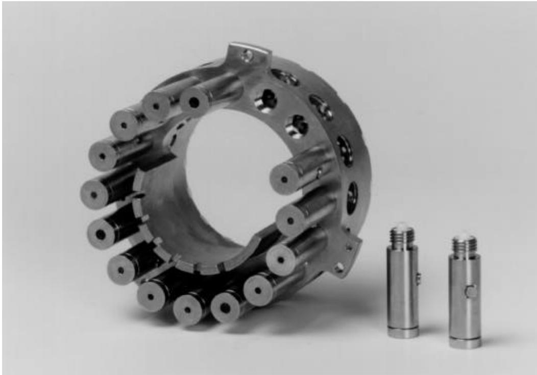
*figure 4* Photograph of the experiment ring with the experiment cells. The windows visible on the outer face of the ring were sealed with a metal insert before the experiment. The drops were observed through the windows on the inner face of the ring.
