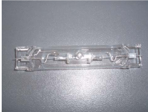
Figure 1.3: A COST reference lamp [22] used for most experiments in this thesis. The burner is made of quartz
