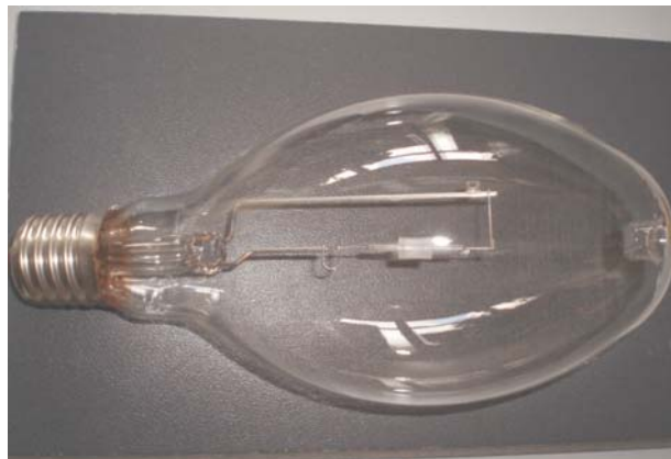
Figure 1.4: One of the lamps used for the XRA experiments. This type of lamp has either quartz COST burners (as in chapter 7) or PCA burners (as in chapter 8 and depicted here). The outer bulb geometry for both chapter 7 and 8 is the same.
