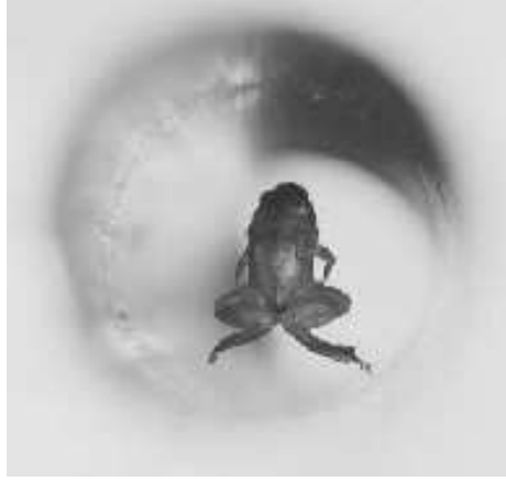
Figure 1.3: A frog levitating in a gradient magnetic field at the HFML, seen from the top.
